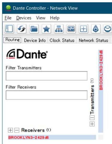
When the Dante module could not be booted in the failsafe mode, it is shown as a fixed Device Name like “Y001-Yamaha-DM3-xxxxxx ” with red text in the network grid view of Dante Controller. In this case, follow the procedure “[Recovery of the Dante module \(without the failsafe mode\)](#)” (page 8) to recover the system.
