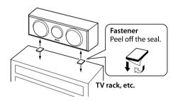
Place the center speaker centrally between the front speakers, facing directly forward.
