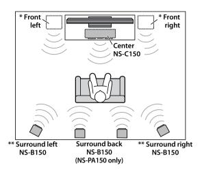
Before you connect the speakers, place each speaker in its respective location. Speaker positioning is very important as it affects the overall sound quality of the system. Place the speakers in locations that will optimize the sound quality at your listening position. Refer to the illustration.
