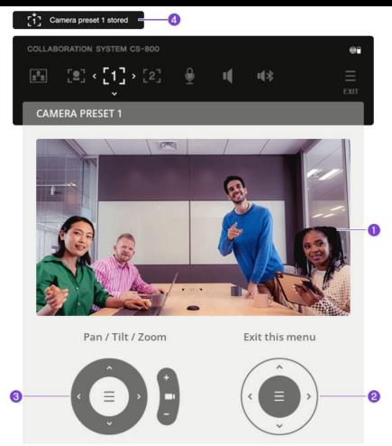
After the [CAMERA PRESET 1] or [CAMERA PRESET 2] screen has been opened, remote control operation is limited to the pan/tilt and zoom buttons. While viewing the live preview screen, use the remote control to adjust the PTZ (pan/tilt/zoom) camera settings.
