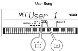
The L (TRACK 1) and R (TRACK 2) indicators light when the respective track contains data. They are unlit when the respective track contains no data. Even if a track contains data, it is unlit when the track is muted. In addition, they flash when the respective track is selected as a Recording target.
