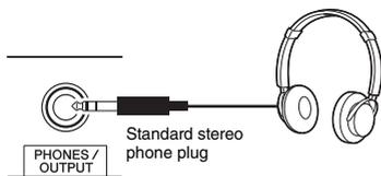
Connect a pair of headphones to the [PHONES/OUTPUT] jack. This jack also functions as an external output. By connecting to a keyboard amplifier, recorder, or other audio device, you can output the audio signal of this instrument to that external device. The speakers of this instrument are automatically shut off when a plug is inserted into this jack.
