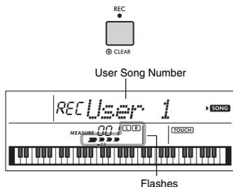
To exit from the Record mode, press the [REC] button again to stop the display from flashing.
