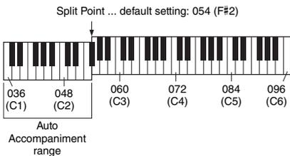
You can change the Split Point via Function number 004 (page 54) by holding down the [ACMP ON/OFF] button for longer than a second.
