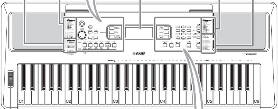
As illustrated, each note of the keyboard has a specific note number and name (e.g., 036/C1), which is used in making various settings, such as Split Point (page 25).
