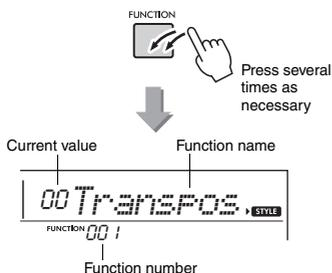
After a few seconds, the Function name may be replaced with the setting value depending on the selected Function.
