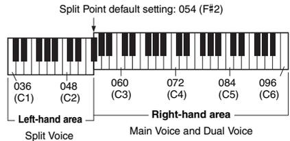
You can play a “Split Voice” in the left-hand area of the keyboard while playing a Main Voice and Dual Voice in the right-hand area of the keyboard. The highest key for the left-hand area is referred to as the “SplitPnt” (Function 004; page 54) which can be changed from the default F#2 key.
