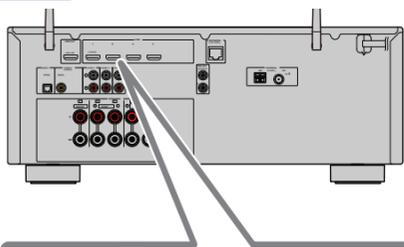
Connect a TV and other sources to the receiver using an HDMI cable (not included). See the receiver's owner's manual for more information.
