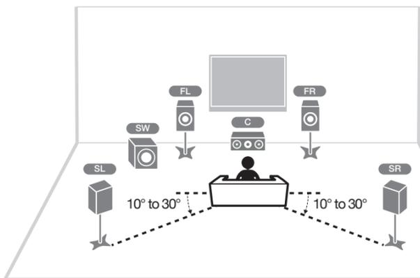
Set up the speakers in the room using the diagram as a reference. The subwoofer may be placed on either side of the front speakers depending on the room layout and personal preference.
