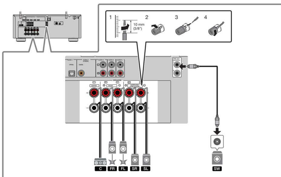
Speaker cables have two wires: one for connecting to the negative (-) terminal of the receiver and speaker, and the other for connecting to the positive (+) terminal.
