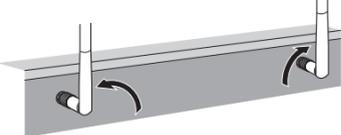
Raise the wireless antennas so that they stand up straight. (Procedures for connecting the unit to a wireless router are described in the owner's manual.) **NOTE:** Do not use excessive force on the antennas – doing so may damage them.
