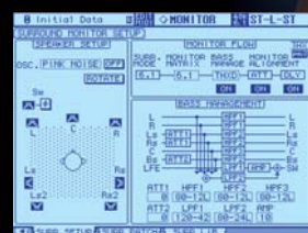
SURROUND MONITOR SETUP (THX pm3™ MONITOR FLOW)
