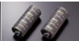
Custom-made 18,000 µF block electrolytic capacitors
