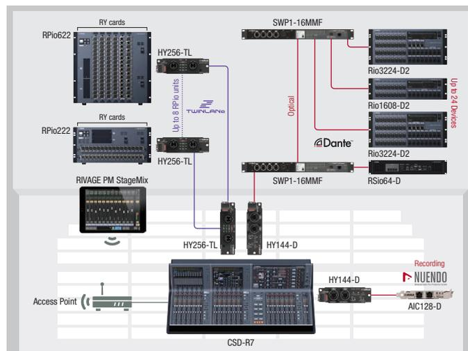
The Rio3224-D2 and Rio1608-D2 can be combined with previous-generation I/O racks in CL/QL based systems, taking advantage of the simplicity and flexibility of Dante networking.
